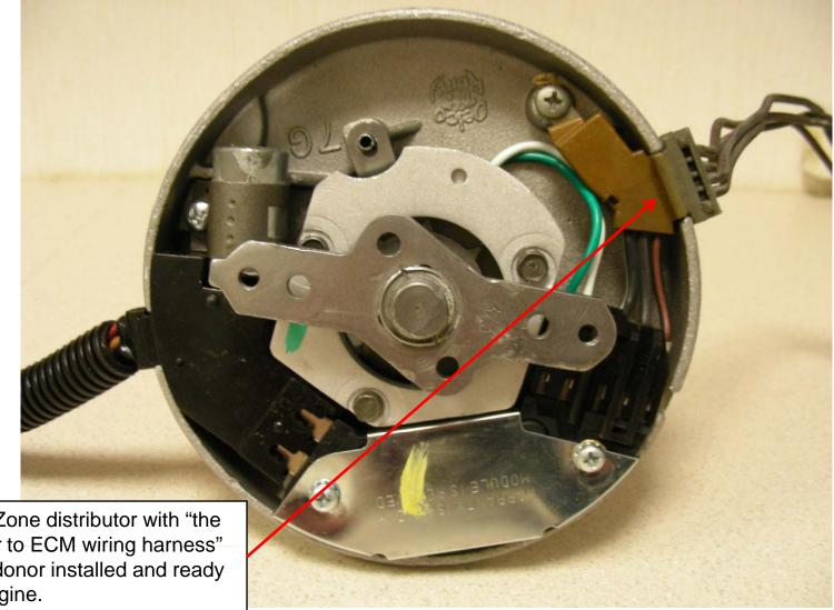
The AutoZone distributor with "the distributor to ECM wiring harness" from the donor installed and ready for the engine.
