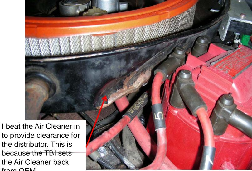
to provide clearance for the distributor. This is because the TBI sets the Air Cleaner back from OEM.
