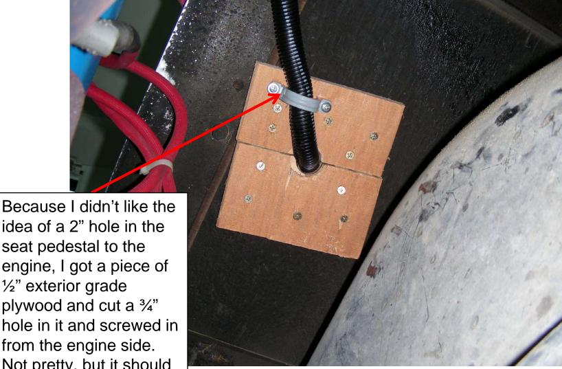
idea of a 2" hole in the seat pedestal to the engine, I got a piece of <sup>1</sup>/<sub>2</sub>" exterior grade plywood and cut a 3/4" hole in it and screwed in from the engine side. Not pretty, but it should work for a while.
