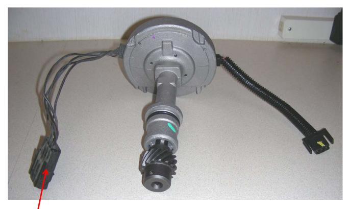
Another view of AutoZone distributor with "the distributor to ECM wiring harness" from the donor installed and ready for the engine.
