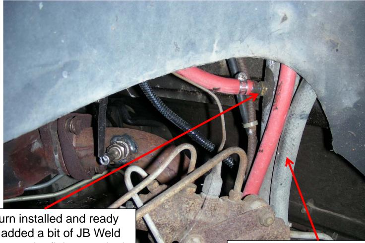
Fuel return installed and ready to go. I added a bit of JB Weld to make sure the fitting was leak free.
