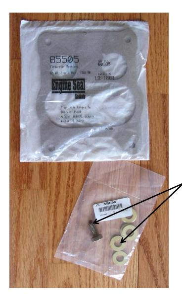
Brass 3/8" washers & stainless steel 3/8"-16x3/4 hex bolt to connect TBI wiring harness ground wires to driver side cylinder head
