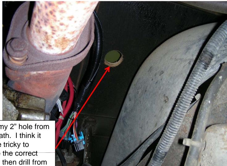
View of my 2" hole from underneath. I think it would be tricky to measure the correct spot and then drill from here.
