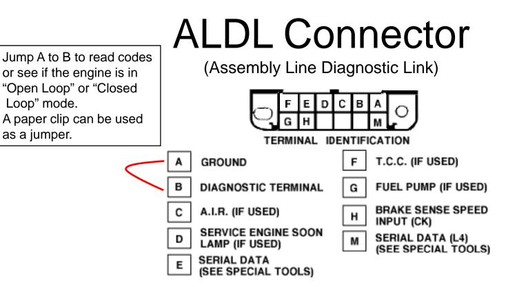
•There should always be a steady "Service Engine Soon" (SES) light when the ignition is "ON" and the engine stopped.
