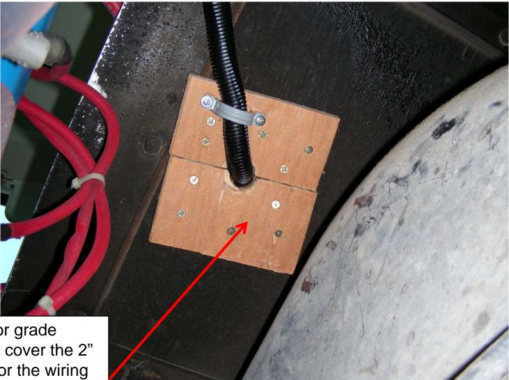
5/8" exterior grade plywood to cover the 2" hole I cut for the wiring harness. I used drywall screws to attach this to
