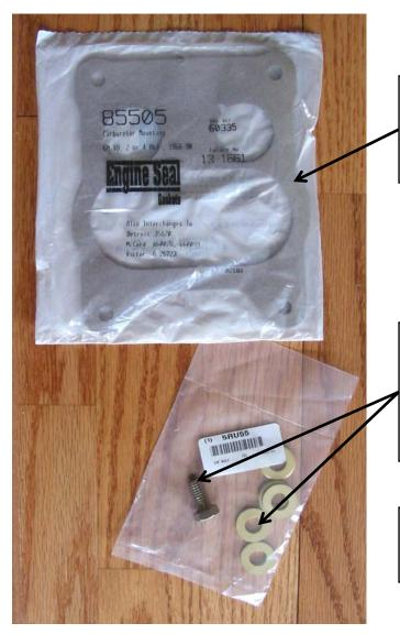
Thick Quadrajet to manifold gasket to replace the thin gasket in Howell's kit.
