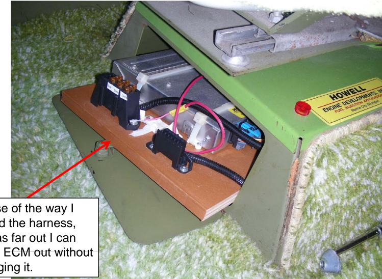
Because of the way I installed the harness, this is as far out I can pull the ECM out without unplugging it.
