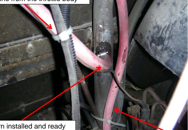
Fuel return installed and ready to go. I added a bit of JB Weld to make sure the fitting was leak free.
