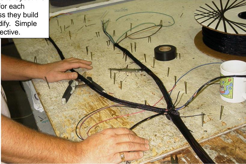
They use boards like this to layout the wires for each harness they build or modify. Simple but effective.
