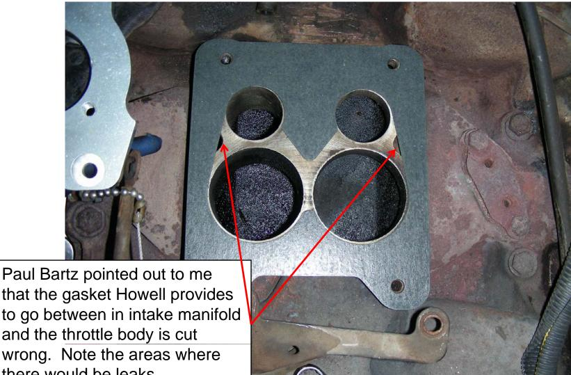
that the gasket Howell provides to go between in intake manifold and the throttle body is cut wrong. Note the areas where there would be leaks.
