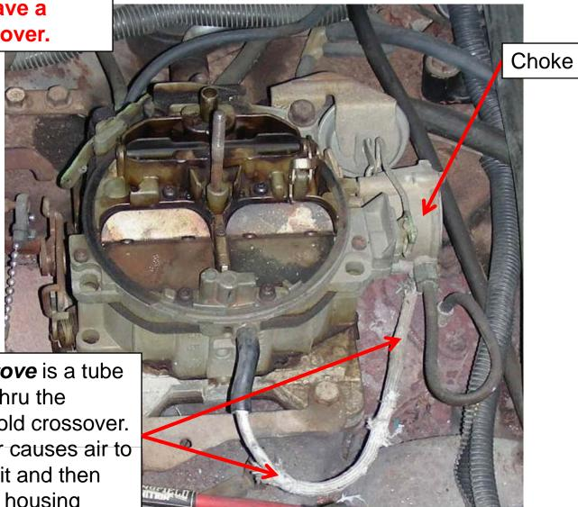
The **Choke Stove** is a tube that is routed thru the exhaust manifold crossover. The carburetor causes air to be drawn thru it and then thru the choke housing
