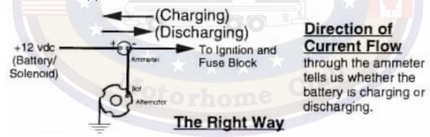
For any of these hook ups, right or wrong, reversing the polarity of the ammeter connections (+ and-) will cause the meter to read backwards and just confuse everything!
