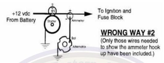
For any of these hook ups, right or wrong, reversing the polarity of the ammeter connections (+ and-) will cause the meter to read backwards and just confuse everything!
